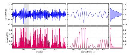
SEAREV is a giant double-pendulum that swings with the waves. An electric generator "brakes" the inner wheel to generates power  $(P_{prod} = T(\Omega) \times \Omega)$ .
